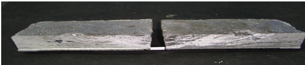
Fig 3(b) Sample with Riser Ø36mmx72mm Height (Plate size, 100mm x100mm x 12.5mm)
