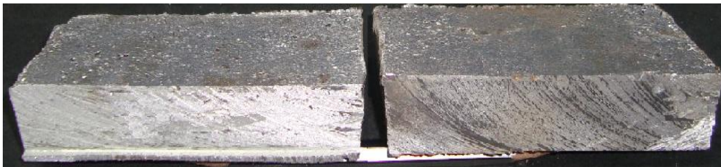
Fig 3(c) Sample with Riser Ø 42mmx84mm Height (Plate size, 100mm x100mm x 25mm)
